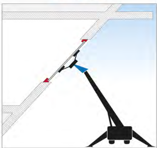
OUTDOOR glazing slanted or Overhead of panes weighing up to 2,500kg with a MANIPULATOR
