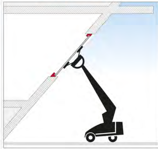
OUTDOOR glazing slanted or Overhead of panes weighing up to 1,000kg with a GLASS ASSEMBLY DEVICE
